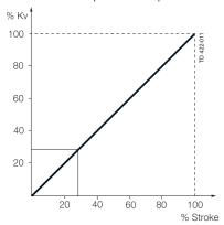
The flow in % of the total flow at a pressure drop of 1 bar.
