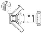
Manual valve: rotate the handle in a clockwise direction to close the valve. Pneumatic valve: shut the air supply to stop the flow of product from the valve. In closed position, the valve body is now ready for sterilization. If steam is used for Sterilization-in-Place, the use of an optional pressure relief valve on the outlet is recommended to ensure proper steam temperature in the valve.
