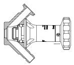
Manual valve: rotate the handle in a counterclockwise direction to open the valve. Pneumatic valve: open the valve by activating the actuator. This retracts the valve stem and membrane seal, which enables the product to flow freely through the open valve.
